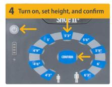
Turn on the device using the power button. Select patient height and press CONFIRM. This sets a size-appropriate tidal volume (TV) and a default respiratory rate. Adult presets default to male. See Table 1 in Section 2b to adjust tidal volume for female patients.
