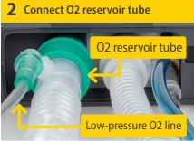
Connect the expandable O2 reservoir tube to the AIR / O2 INTAKE port.
